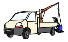
Vehicle mounted loading cranes are handy when you have to take large machines to the jobsite on the back of your truck.
